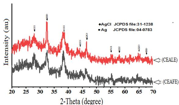
**Fig. 2:** X-ray diffraction pattern of AgNPs from *C. equisetifolia* aqueous leaves extract (CEALE) and aqueous fruits extract (CEAFE)
